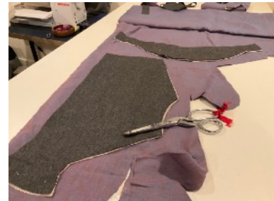
Top fabric and foundation laid on lining before cutting
